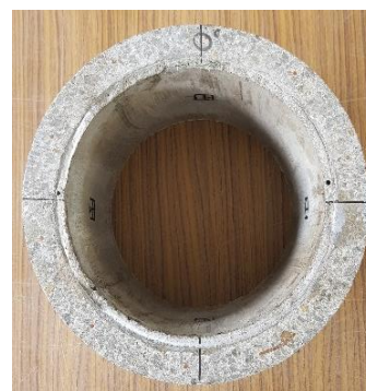
Fig.3 Pipe after Rehabilitation
